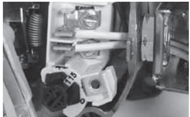
Figure 11: Voltage set to 115 volts, Dial Type
